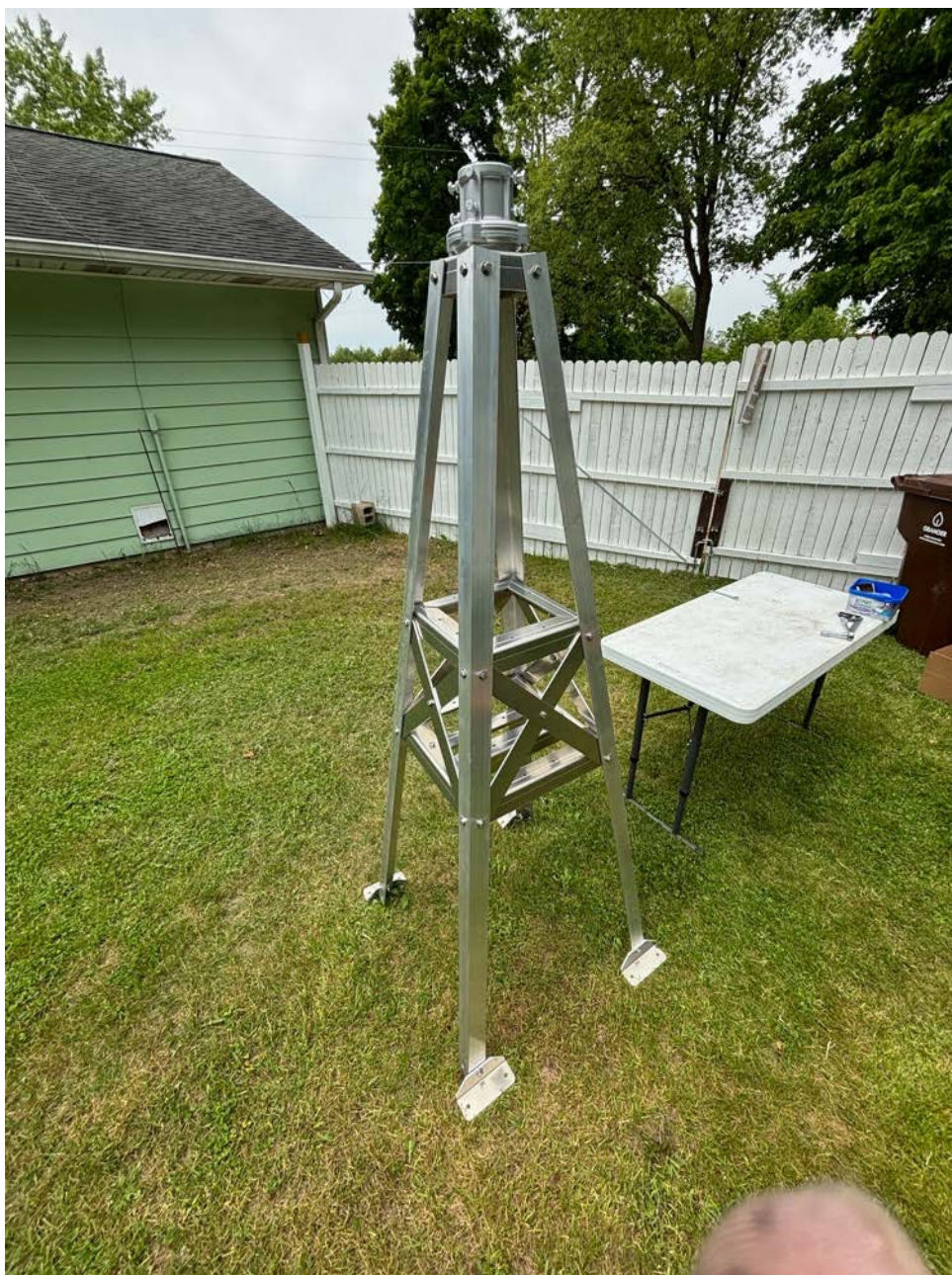
Figure 13 The finished 610HD Roof Tower Assembly.
